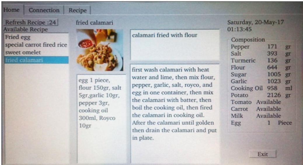
Figure 9. LCD displayed the recipe according to the availability items either in smart refrigerator or smart food cabinet
